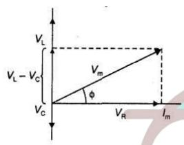
From the diagram, we observe that the vector sum of the voltage amplitudes  $V_R$ ,  $V_L$ , and  $V_C$  equals a phasor whose length is the maximum applied voltage  $V_m$ , where the phasor Vm makes an angle  $\varphi$  with the current phasor Im. Since the voltage phasors,  $V_L$  and  $V_C$  are in opposite direction, therefore, a difference phasor  $(V_L - V_C)$  is drawn which is perpendicular to the phasor  $V_R$ . Adding vectorially we have
